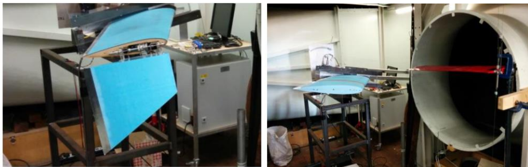
Figure 1.14. (a) Folding wingtip device, (b) Gust excitation test [81]
